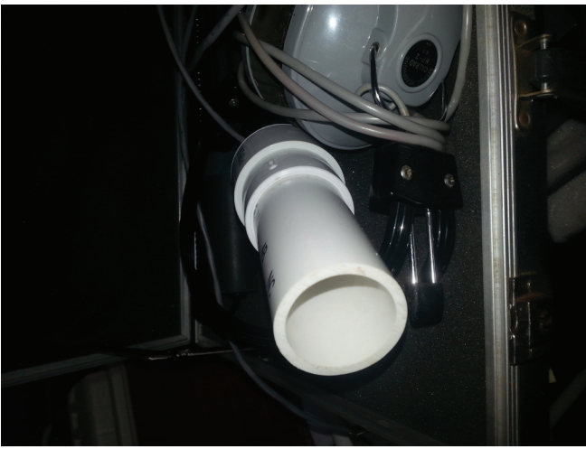
Fig. 3: Homemade ultrasonic hand probe.
