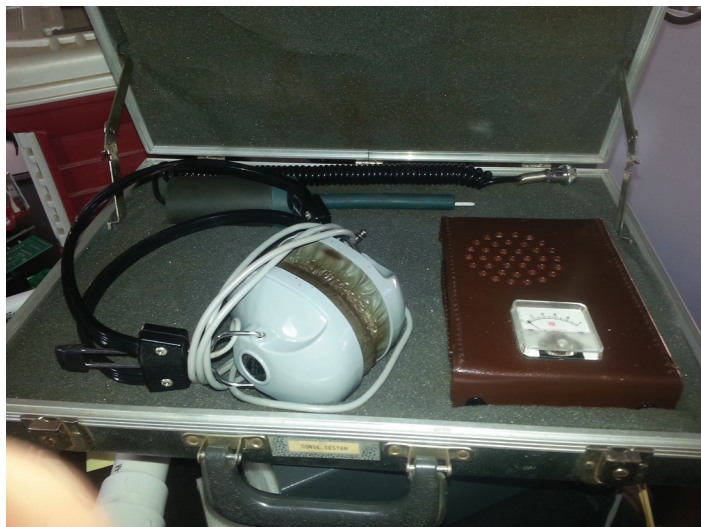
Fig. 2: The ultrasonic detection kit which was purchased as the foundation of my arcing RFI location system.
