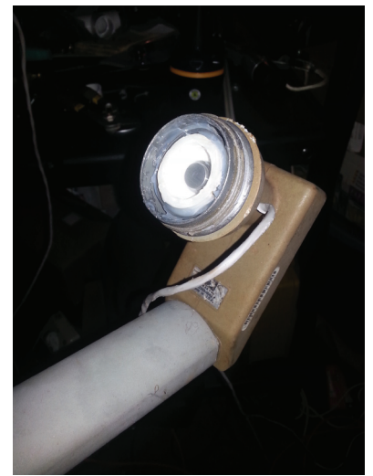
Fig. 4: Modified feedhorn/LNB with ultrasonic transducer installed.
