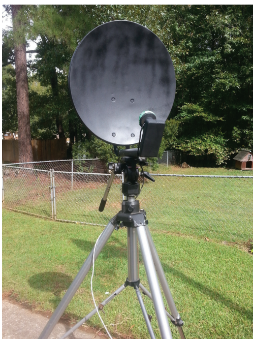
Fig. 5: Completed directional ultrasonic reflector, with a couple of coats of black paint applied.
